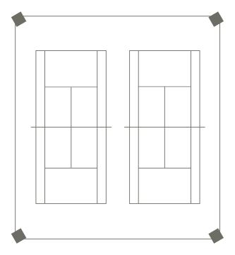
Both corner and side-lighting systems can and should be designed and installed to meet Australian Standards AS2560 Guide to Sports Lighting and AS2560.1 - Part 1 General Principles and AS2560.2.1 - Part 2.1 Lighting for Outdoor Tennis for design luminaries, z levels, uniformity and pole heights.
