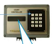
TIP: The Controller display will switch off 5 minutes after the controller has been activated. Press any key to switch the display on and activate the keypad.
